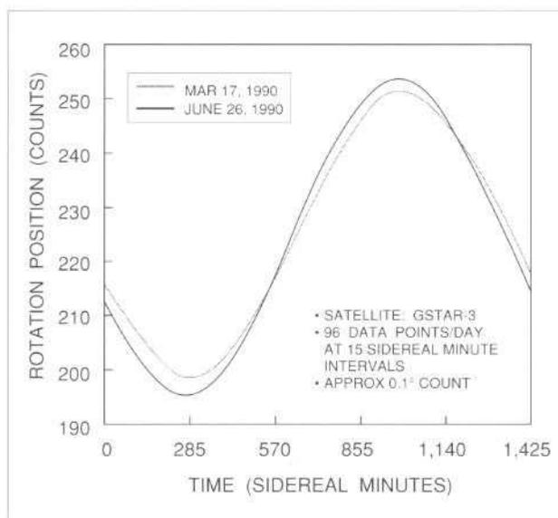
Figure 9. Pedestal drive positions showing tracking of the increasing satellite inclination
