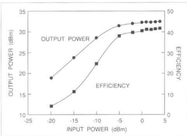
Figure 3. Optimized amplifier offering better than 2-W output power and 43-percent efficiency
