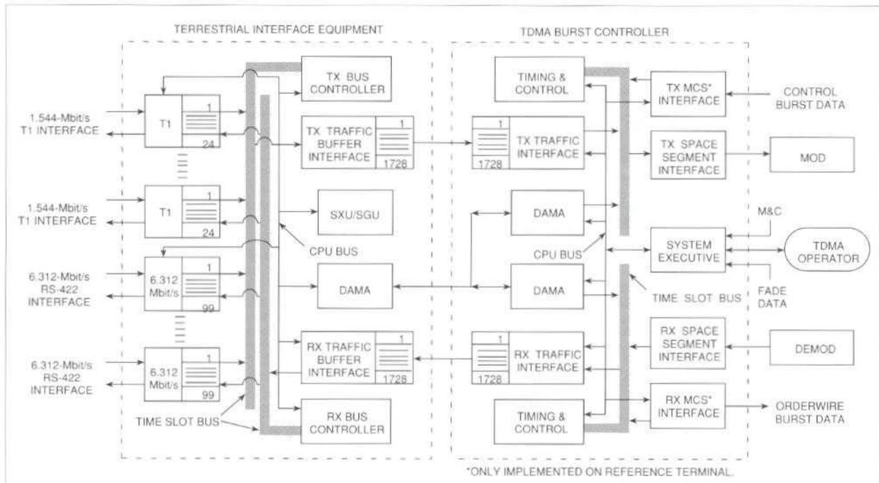
Figure 2. TDMA terminal functional architecture
