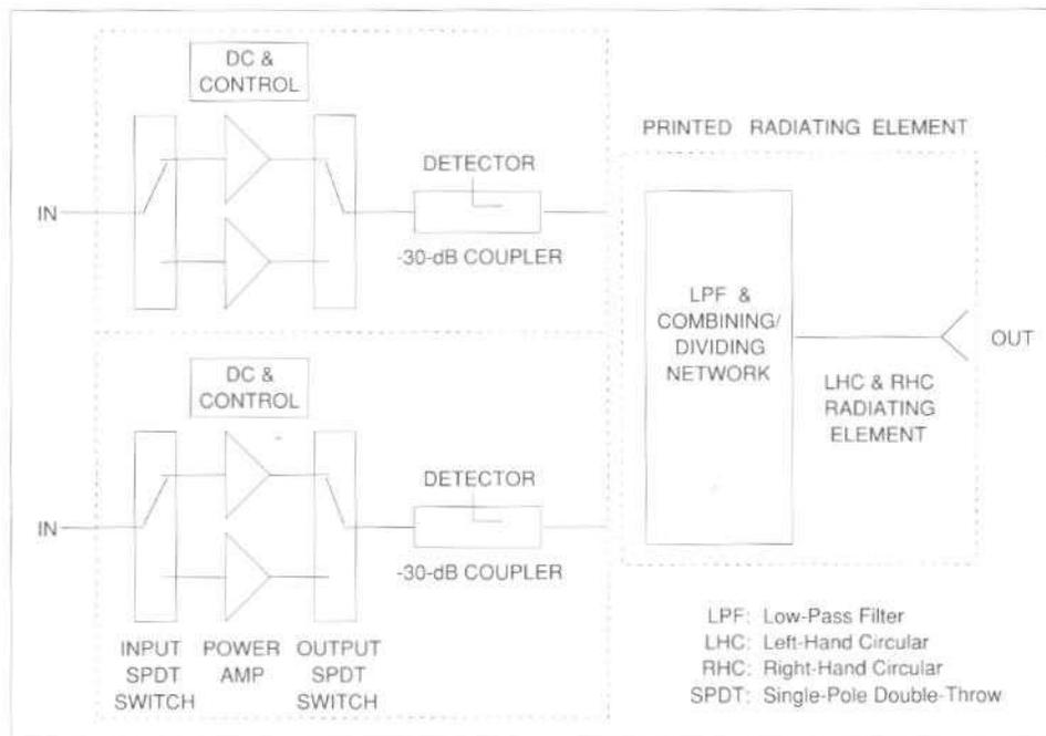
Figure 7. Active circuit module showing MMIC components, redundancy, and monitoring capability
