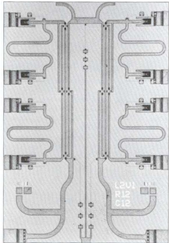
Figure 12. GaAs MMIC analog phase shifter based on ion-implanted varactor diodes
