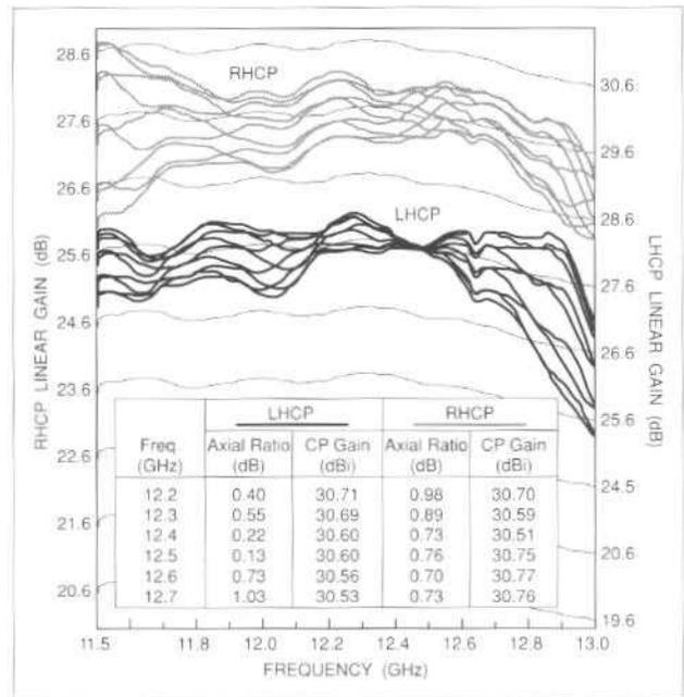
Figure 13. Measured axial ratio data showing good discrimination between two circularly polarized beams
