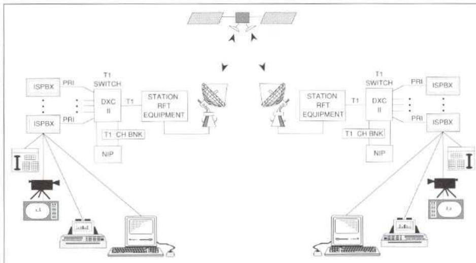
Figure 4. Pilot system for a satellite-based private ISDN uses a NIP for management functions
