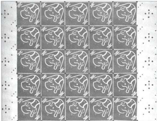
Figure 4. A breadboard 25-element array model used to simulate performance of the full array
