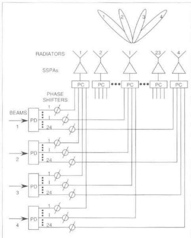
Figure 1. Ku-band, high-power, phased-array antenna concept to provide independent steerability for multiple beams
