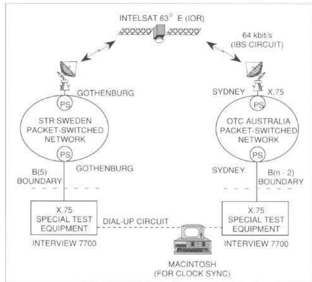
Figure 5. High-speed packet-switched QOS experiment configuration will test QOS parameters over 64-kbit/s links
