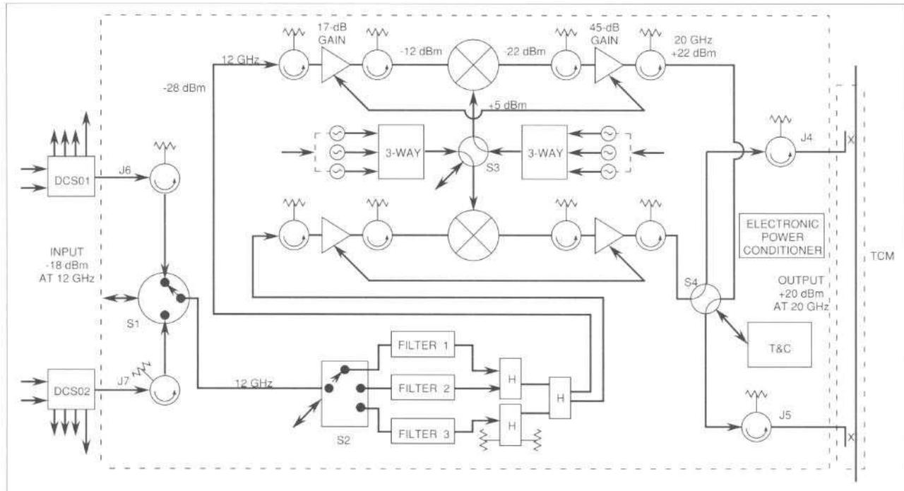
Figure 16. Block diagram of ITALSAT IOTT which provides bypass capability during in-orbit testing
