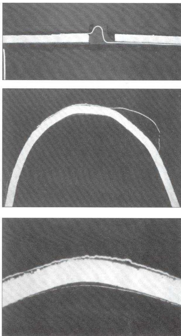
Figure 13. Cross sections of an INTELSAT VII solar cell interconnect exposed to atomic oxygen during a Space Shuttle flight
