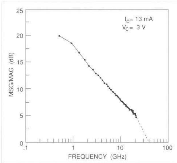
Figure 9. Microwave performance of  $2.5 \times 30\text{-}\mu\text{m}$  HBT
