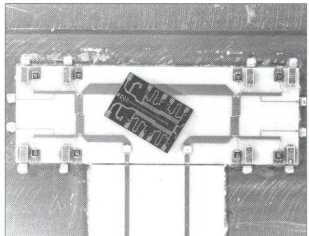
Figure 10. MMIC analog phase shifter shows considerable size reduction compared to its MIC counterpart
