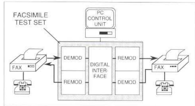
Figure 9. Facsimile test set permits real-time manipulation of facsimile protocols in the presence of various impairments
