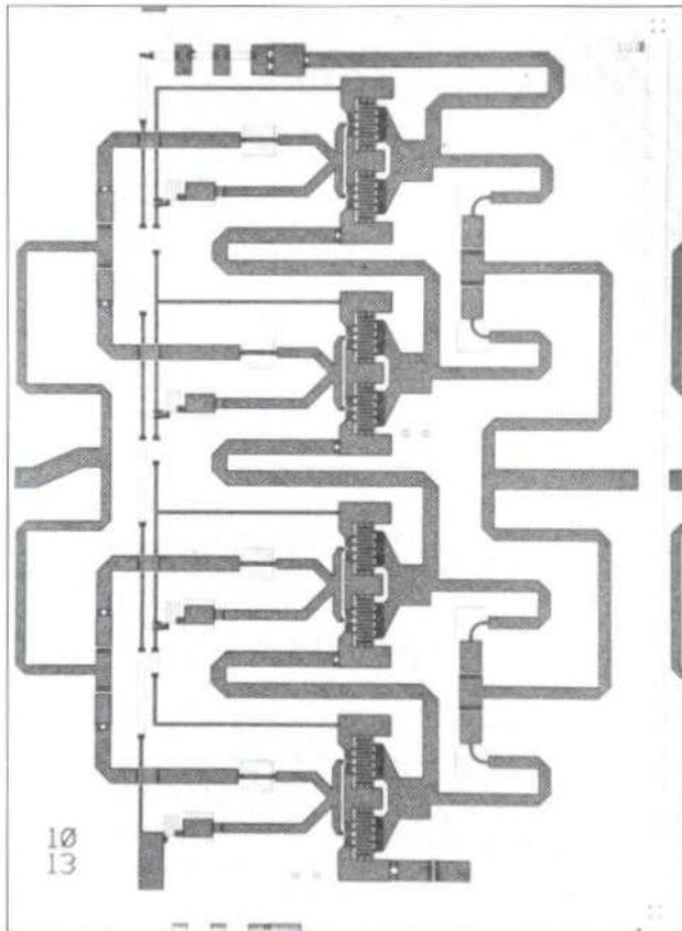
Figure 4. Four-stage MMIC designed to operate at 30-W bias
