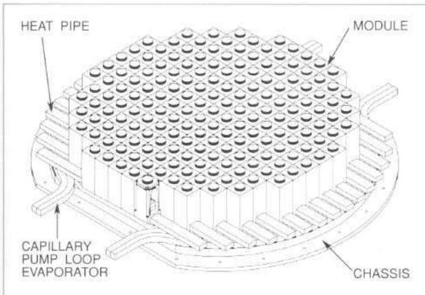
Figure 5. C-band, 177-element active array emphasizing modularity and light weight
