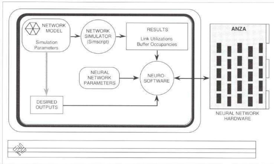
Figure 11. Simulated environment for network training was implemented on a SUN workstation
