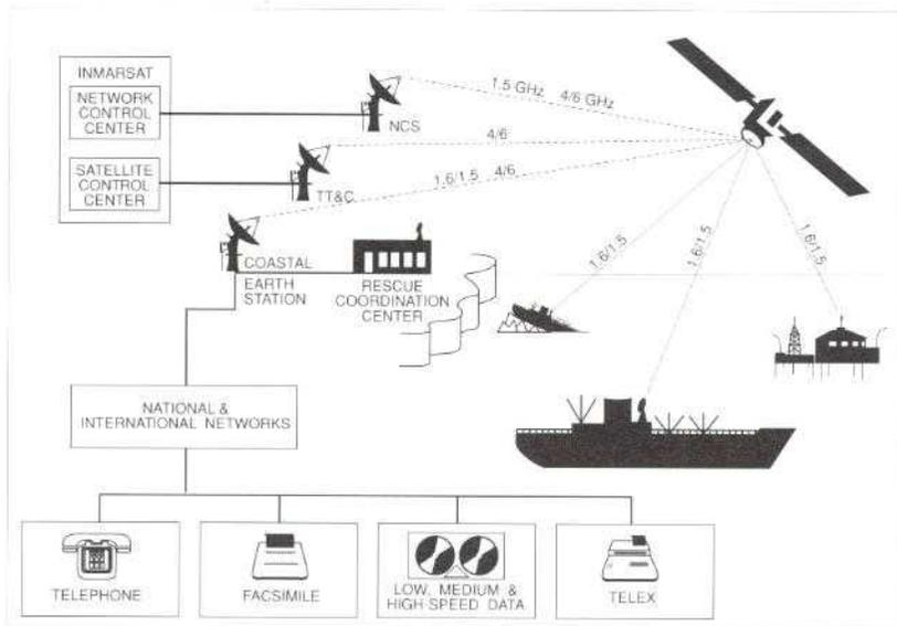
Figure 5. Overview of the Inmarsat-B system that is being developed to replace the analog Inmarsat-A system
