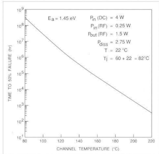
Figure 11. Reliability test results for COMSAT power-MESFET-based MMICs
