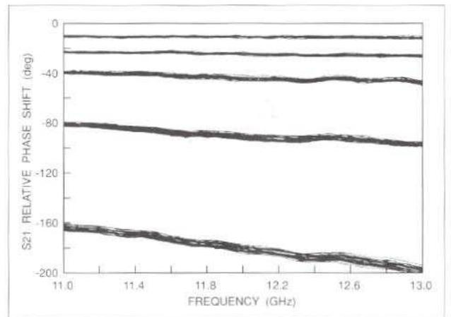
Figure 3. MMIC phase shifters provide uniform and reproducible phase performance of the BFM shelf
