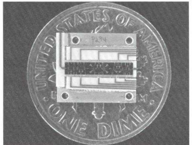
Figure 2. Miniaturized MMIC phase shifter forms a key building block of the beam-forming matrix
