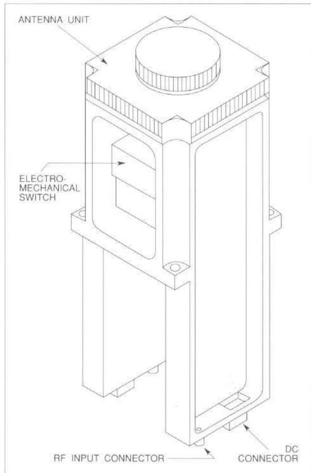
Figure 6. Single module with patch antenna and MMICs forms a basic building block of the C-band array
