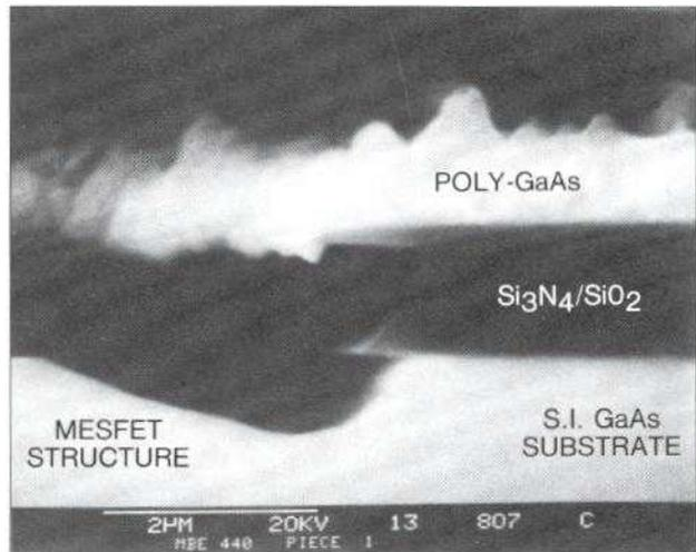
Figure 5. SEM of a T-gate created using COMSAT's improved process
