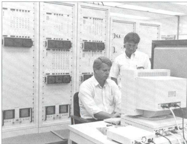
Figure 3. 110-Mbit/s TDMA equipment under test
