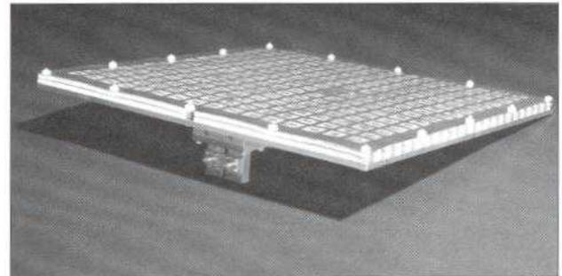
Figure 12. Flat-plate antenna capable of receiving two circularly polarized beams
