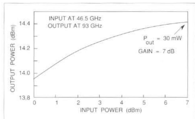
Figure 15. W-band MMIC doubler/amplifier chain delivers high power and gain for missile/transceiver applications
