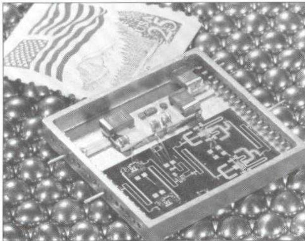
Figure 2. Demonstration amplifier using silicon motherboard technology
