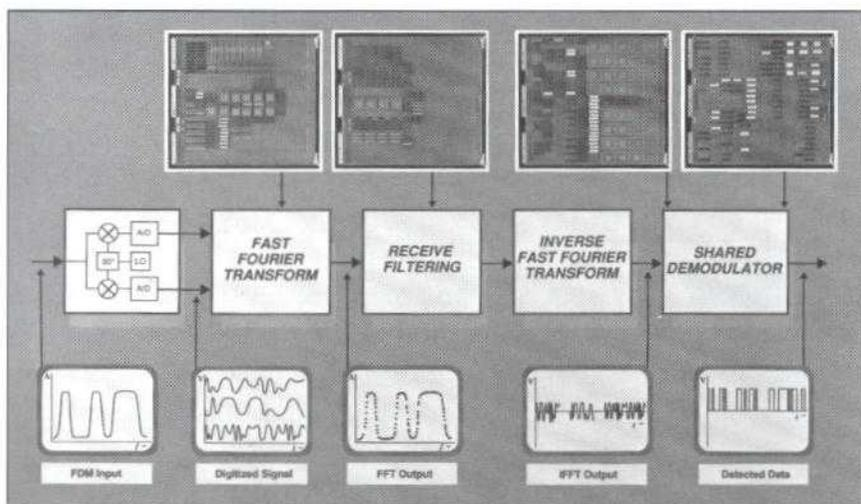
Figure 4. POC on-board multicarrier demultiplexer/demodulator is intended to reduce system mass and power
