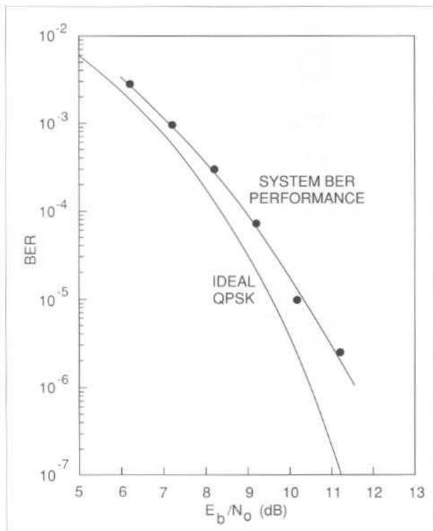
Figure 5. BER performance of 2-Mbit/s carrier after processing
