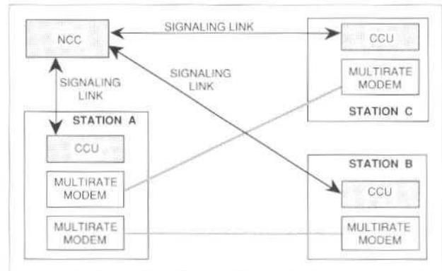
Figure 13. Architecture for a demand-assigned IBS system demonstrated at a field trial in Clarksburg, Maryland
