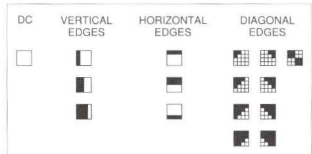
Figure 2. Perceptually important image patterns in a  $4 \times 4$  block
