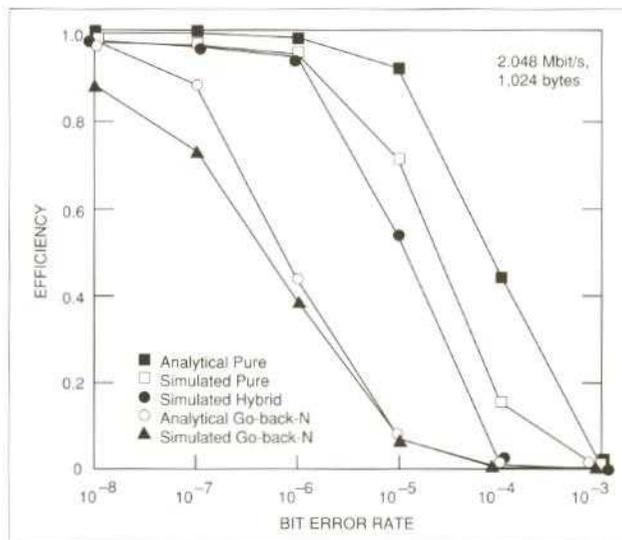
Figure 3. Throughput efficiency can be improved by using a selective retransmission scheme
