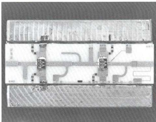
Figure 11. A low-cost, two-stage LNA for integration in the flat-plate antenna
