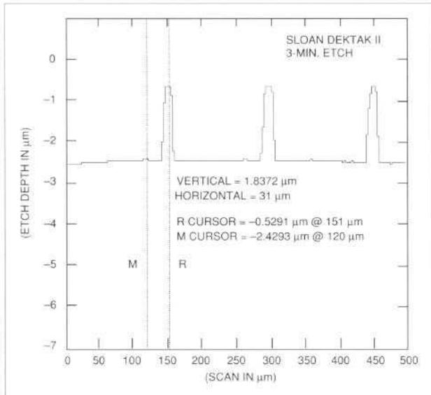
Figure 8. DEKTAK profile of RIE channels etched in the core layer of two-layer polymer films spun on silicon wafer; photoresist optically exposed using image mask; channel filling by buffer completes waveguide fabrication
