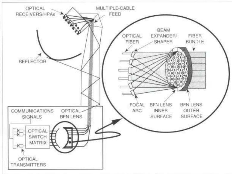
Figure 6. Possible deployment architecture for optical space-fed BFN on board satellites features light weight and small size
