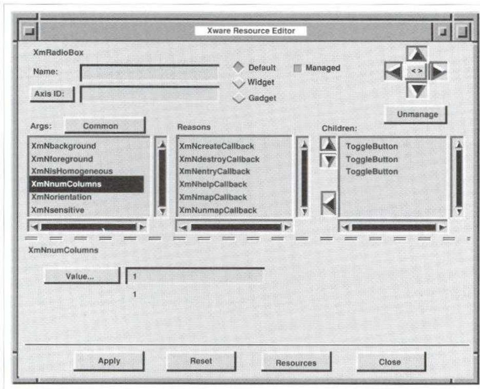
Figure 2. XWARE resource editor screen allows users to design and modify screens for their specific applications
