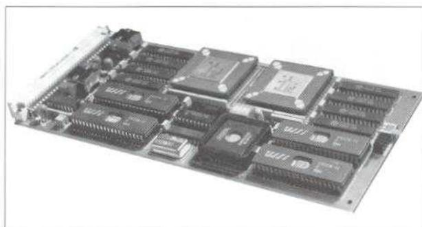
Figure 6. COMSAT's 4.8-kbit/s CELP speech codec
