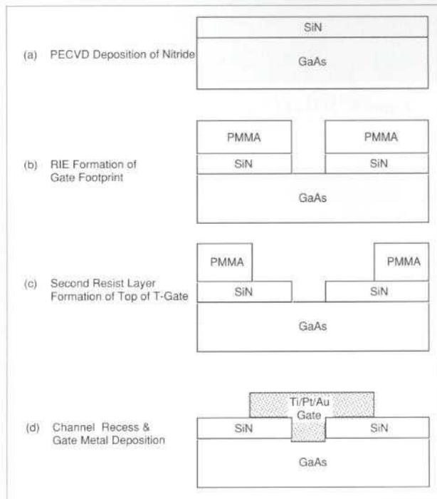
Figure 6. COMSAT's improved T-gate fabrication process
