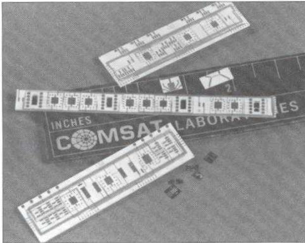
Figure 1. Microwave circuit components for Ku-band antenna
