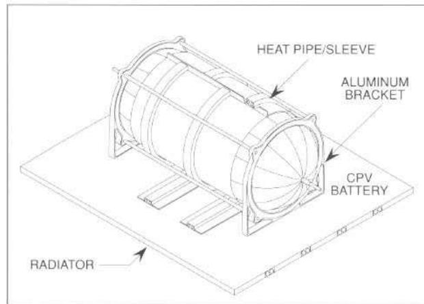
Figure 4. CPV battery mount is a lightweight, rigid support structure that provides good heat transfer
