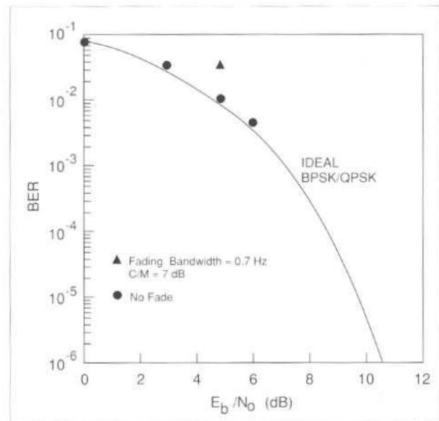
Figure 10. BER performance of the Laboratories' preambleless signaling channel demodulator (production version) (random frequency offsets:  $\pm 1,450$  Hz, Doppler period: 48 s, adjacent channel interference: none)
