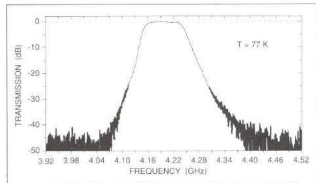
Figure 2. COMSAT-designed four-pole filter features resonator Q of approximately 5,000.
