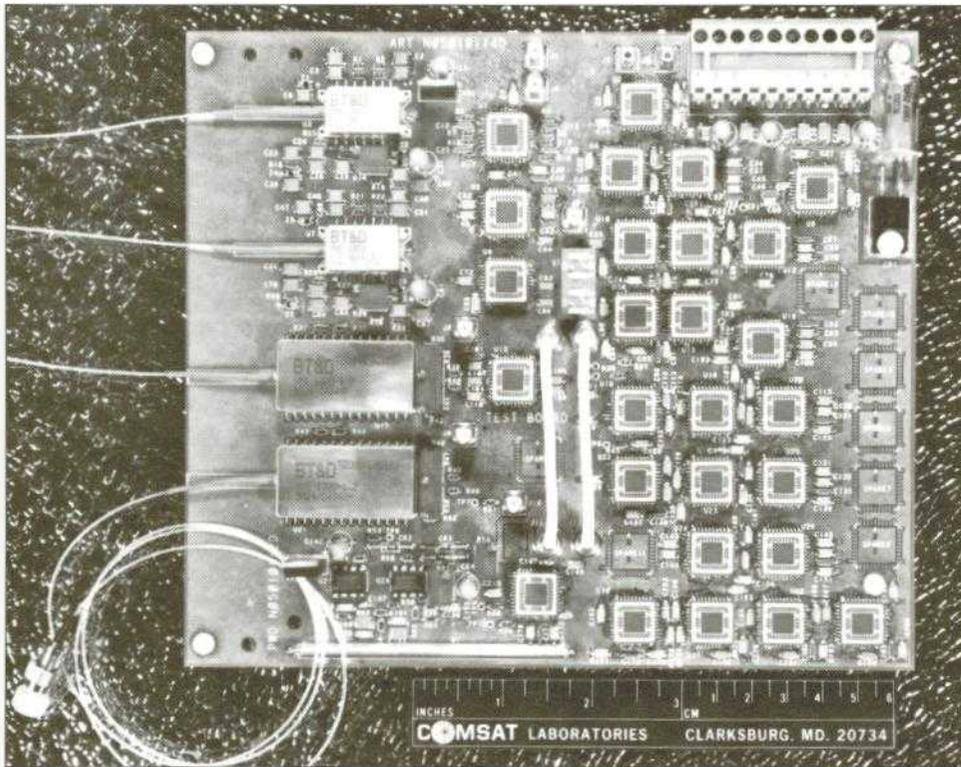
Figure 2. Modular baseband switch reduces earth station cost and complexity
