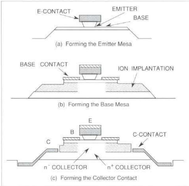
Figure 8. HBT cross sections showing steps in COMSAT's unique fabrication process
