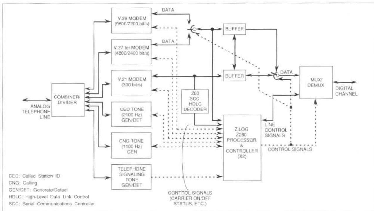
Figure 11. Facsimile interface unit functionality has been implemented in hardware
