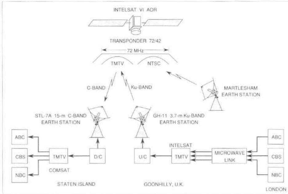
Figure 1. TMTV technology was demonstrated in a transatlantic field test
