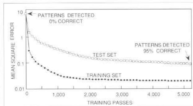
Figure 10. Neural networks can easily be trained to detect patterns
