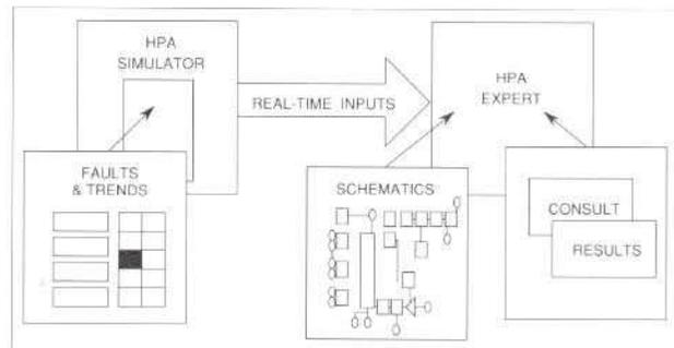
Figure 8. HPA expert system receives simulated real-time data from monitoring instruments
