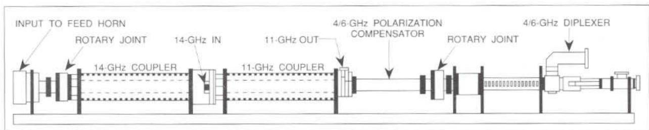
Figure 8. Dual-band earth station antenna feed capable of operation at C- and Ku-band up-links and down-links
