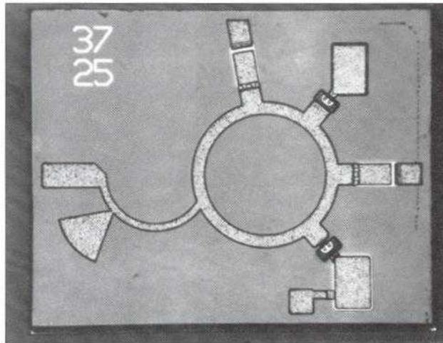
Figure 16. W-band monolithic mixer chip for seeker/transceiver systems
