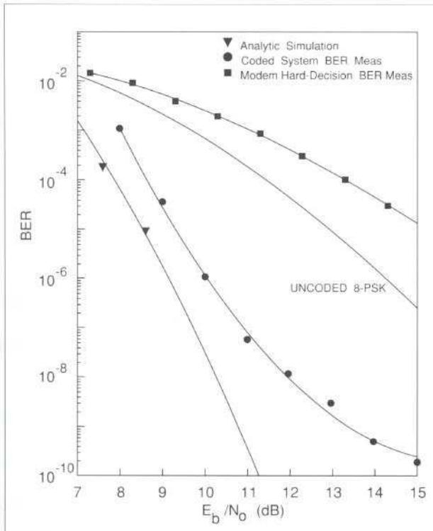
Figure 7. System performance test results
