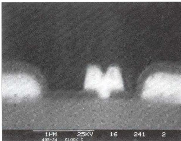
Figure 7. Cross section of the T-gate
