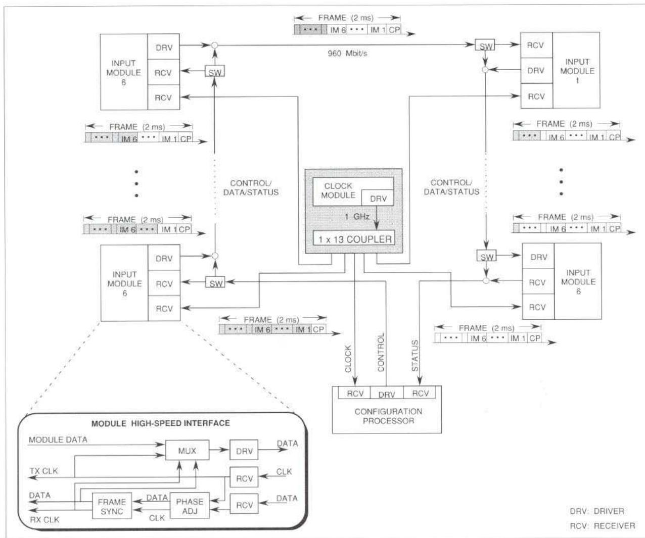
Figure 1. Regenerative ring with star-coupled clock distribution will handle a total throughput of 1 Gbit/s
