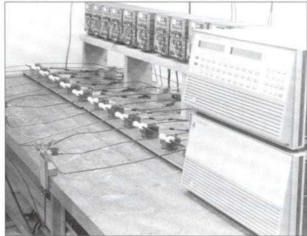
Figure 10. GaAs MMIC RF-biased life test system with individual dynamic temperature control
